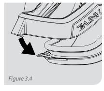
Close the visor making sure it <u>LATCHES</u> <u>SECURELY</u> to the front of the jaw. Listen for the visor latching over the tab on the front of the jaw.
