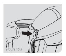
Line up the Welding Visor connection sockets with the Pivot Pins on the Z-LINK and insert them into the Z-LINK until they snap in securely. This can be done while wearing the Z-LINK.
