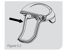
Starting from on of the top corners, insert the new visor seal by pressing the edge into the track all of the way around the visor opening.
