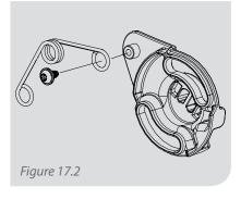
Position the spring onto the new flip up mechanism and secure it with the screw provided.
