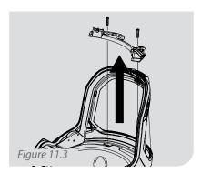
To remove the Impact Liner, remove the head harness bracket by removing the screws holding it in place.
