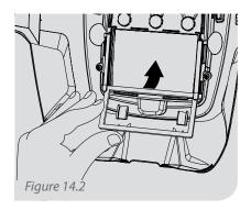
To install the magnifying lens for welding, slide the lens up into the brackets at an angle until it is securely in the brackets.
