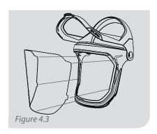
To attach the Visor, insert the selected Safety Lens into the inner visor and secure the inner and outer visors together.
