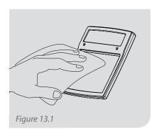
Once removed, the ADF can be cleaned with a soft tissue or a cloth soaked in mild detergent (or alcohol).
