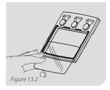
To replace the Rear ADF Lens, slide the lens out and replace it with a new one.
