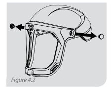
Remove the cap, pivot pin, and spring from the visor on both sides. Pull the visor out of the pivot points and remove from the helmet.
