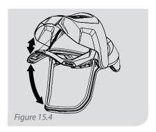
The Welding Visor can be rotated up independently of the Visor or together with the Visor.
