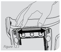
Push the tabs inside the weld visor apart to release the ADF Retainer.
