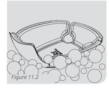
The comfort pad can be washed with mild detergent or replaced.
