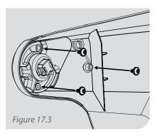
Carefully align the replacement spring and the flip-up mechanism onto the pegs in the Welding Visor. Insert and screw in the 3 replacement screws to attach the spring and mechanism without over tightening.
