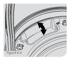
Airflow can be directed by positioning the air flow director so that the air flows more towards the visor or towards the face.
