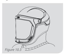
When using a face seal, make sure the elastic edge is under the users chin at the front and is in contact all of the way around the neck and back of the head.
