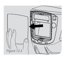
Remove the Impact Lens by squeezing together the sides of the Impact Lens. If just replacing the Impact Lens, then place the new Impact Lens in and replace the green ADF Retainer.
