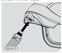
Insert the threaded end of the breathing tube (04-835) into the threaded hole in the back of the Z-LINK and screw the breathing tube in completely without over tightening.
