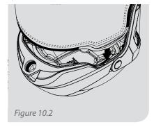
Then press the rubber trim on the cape or face seal into the track that goes around the underside of the helmet, making sure the cape/face seal is completely attached all of the way around.
