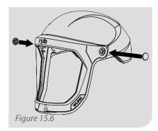
If the Welding Visor is not going to be used again for a while, the socket caps can be snapped back into the Pivot Pins to keep the area free of debris.
