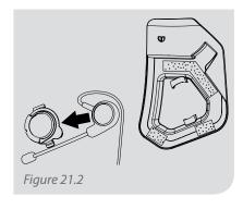
Place the Communication ear piece into the attachment clip. Then attach the Communication Cip into the slots on the inside of the cover.
