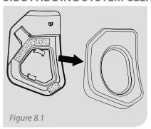
Remove the side pads from the covers that are attached with velcro.
