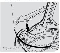
To install the cape or face seal, start by attaching the cape clips on the sides of the cape. Make sure the clip goes over the notch on the helmet and the clip edge goes into the track around the edge of the helmet.
