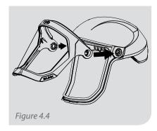
Place the visor onto the helmet pivot points, insert the pivot pins and springs, then screw in the attachment screws from the inside of the helmet until tight.
