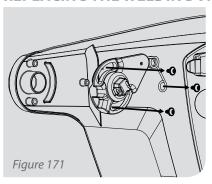
The flip-up mechanisms and springs can be replaced if needed. Using a small screw driver, remove the three screws that hold in the mechanism being careful to not strip the plastic they are threaded into.
