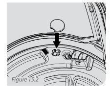
Insert the caps into the holding sockets on the Head Harness Bracket so they don't get lost while using the Welding Visor.
