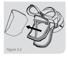
Pull out the lens and insert a new Safety Lens making sure the tabs of the lens are in all four attachment points on the visor and the lens is inside of the guide along the bottom front edge of the visor.
