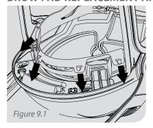
To remove the brow pad, stretch the brow pad over the hooks on the head harness and take it off. Clean it with mild detergent or replace it with a new one.
