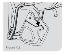
Slide the ends of the head harness into the slots on the side pad covers.
