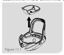
The comfort pad is attached to the inside of the Impact Liner with velcro. Pull the comfort pad out of the helmet.
