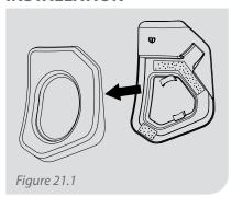
Remove the side pad from the cover that is attached with velcro on the side of the helmet that the Communication is to be installed. The Communication can be installed on either side of the helmet.
