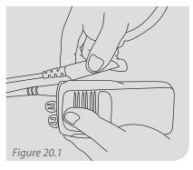
Connect the PTT Cable to the Hand Set depending on the type used.
