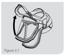
To replace the Safety Lens, lift up the visor, unlatch the inner visor from the outer visor and open them apart.
