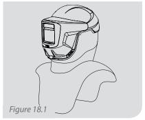
When welding, be sure to install a approved RPB® welding cape for adequate protection from sparks, debris, and light flashes. Follow the cape installation instructions on page 16.
