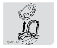
Rotate the Impact Liner out of the helmet shell. The inside of the shell can be wiped with mild liquid detergent or a cleaning wipe.
