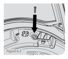
The position of the head harness can be adjusted by loosening the screws that hold the front bracket and sliding it forward or backwards into the desired slot. Once in position, tighten the screws.
