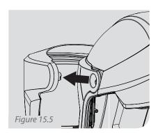
To remove the Welding Visor from the Z-LINK, pull the sides of the Welding Visor out until the connection sockets snap out of the Pivot Pins in the Z-LINK. This can also be done while wearing the Z-LINK.
