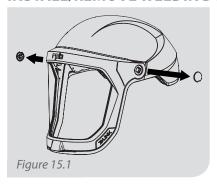
To install the Z-LINK Welding Visor, remove the pivot pin caps on the Z-LINK.
